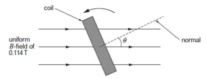
The flux **linkage** of the coil for the angles  $\theta = -5^{\circ}$  and  $\theta = +5^{\circ}$  is 1.29 Wb turn in each case.
