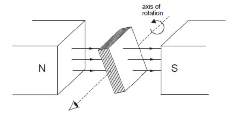
This second diagram is a 2D representation of the coil looking along the axis of rotation.
